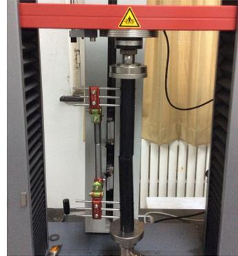
**Fig. 3.** Experimental testing of novel fixator under compression load
