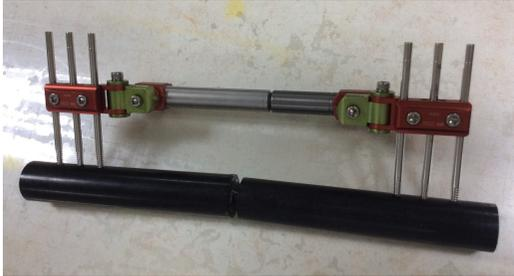
**Fig. 2.** A novel external fixator with fragments apart
