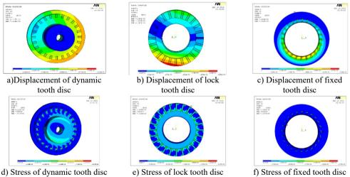
Fig. 4. Equivalent displacement and Equivalent stress diagram
