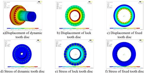
Fig. 3. Equivalent displacement and Equivalent stress diagram
