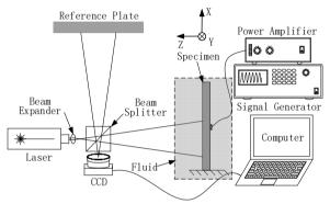
Fig. 1. Schematic of out of plane movement detection system
