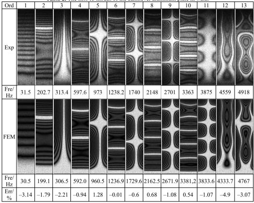
Table 2. The first 13 modes of the cantilever aluminum plate in water
