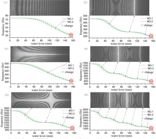
Fig. 5. Influence of different water levels on the first 6 natural frequencies of cantilever plates
