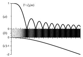
Fig. 2. Variation of gray-value with vibrating amplitude: a) zero-order Bessel function, b) first-order bending fringe pattern of cantilever beam, c) first-order bending mode of cantilever beam
