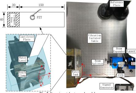
Fig. 3. Experimental setup and model
