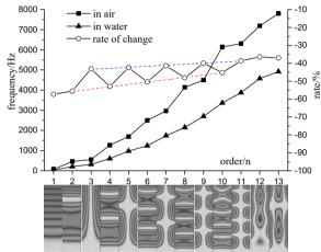
Fig. 7. Comparison of the first 13th order wet and dry modal frequencies of cantilever plate
