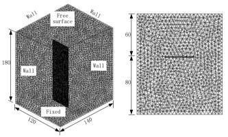
Fig. 4. Fluid-structure coupled finite element model
