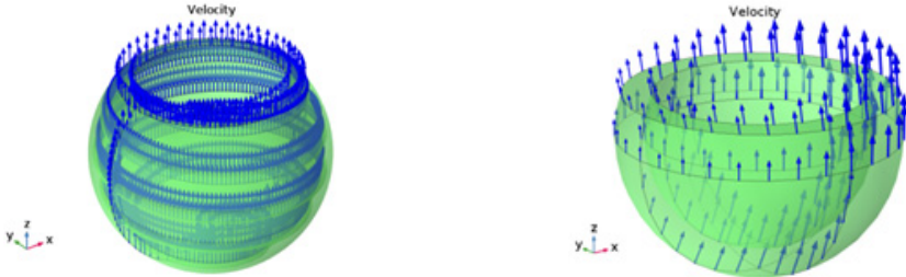
a) Film velocity vector with spiral groove b) Film velocity vector without spiral groove Fig. 9. Oil film velocity vector distribution
