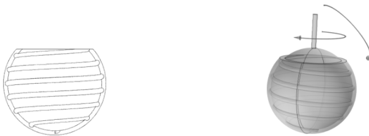
Fig. 2. Schematic diagram of spiral groove structure of spherical bearing of 3-DOF motor
