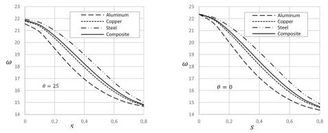
Fig. 3. Frequency versus crack depth ratio with and without temperature
