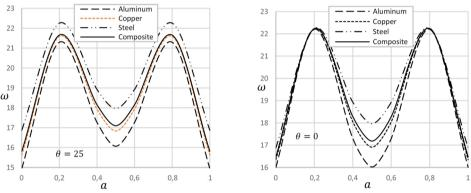
Fig. 5. Frequency versus crack location with and without temperature
