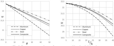
Fig. 2. Frequency versus change of temperature and length to height ratio
