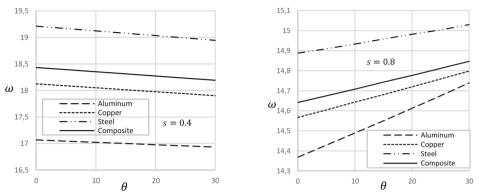
Fig. 4. Frequency versus change of temperature for different crack depth ratios
