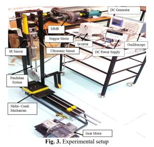
The tuning pendulum arm is attached to a shaft, which is in turn mounted on two ball bearings (bearing diameter,  $r_b = 12$  mm) to the supporting frame. A four-phase stepper motor (NEMA 23) with a maximum torque 3 N.m is attached at the pendulum's tip and enables automatic adjustment of the pendulum length.
