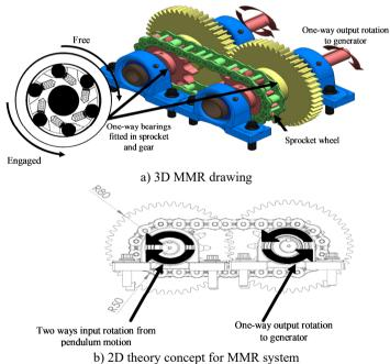
Fig. 4. Working principle of MMR
