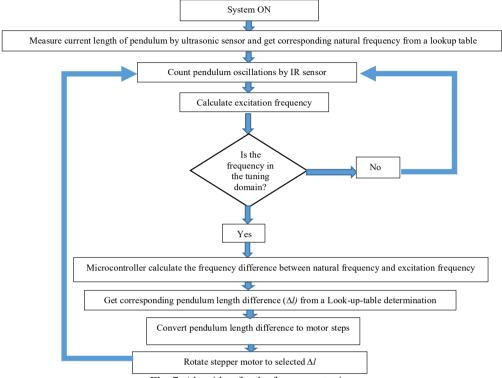
Fig. 7. Algorithm for the frequency tuning
