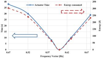
Fig. 11. Energy consumed by the actuator and the time taken for the device to recover the energy
