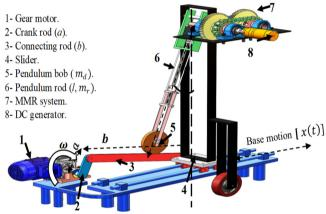
Fig. 1. Schematic pendulum-shaker system
