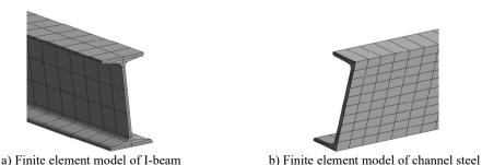
Fig. 5. Finite element model of the section steel
