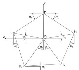
**Fig. 3.** The scheme of the bore centers in the plane of the carrier cheek *YZ* (*P*) and angular values for trigonometric ratios ( $\alpha$ )
