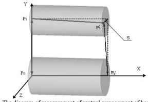
Fig. 1. The diagram of measurement of mutual arrangement of bores for axle of the first satellite pinion relatively to the central axis of the carrier
