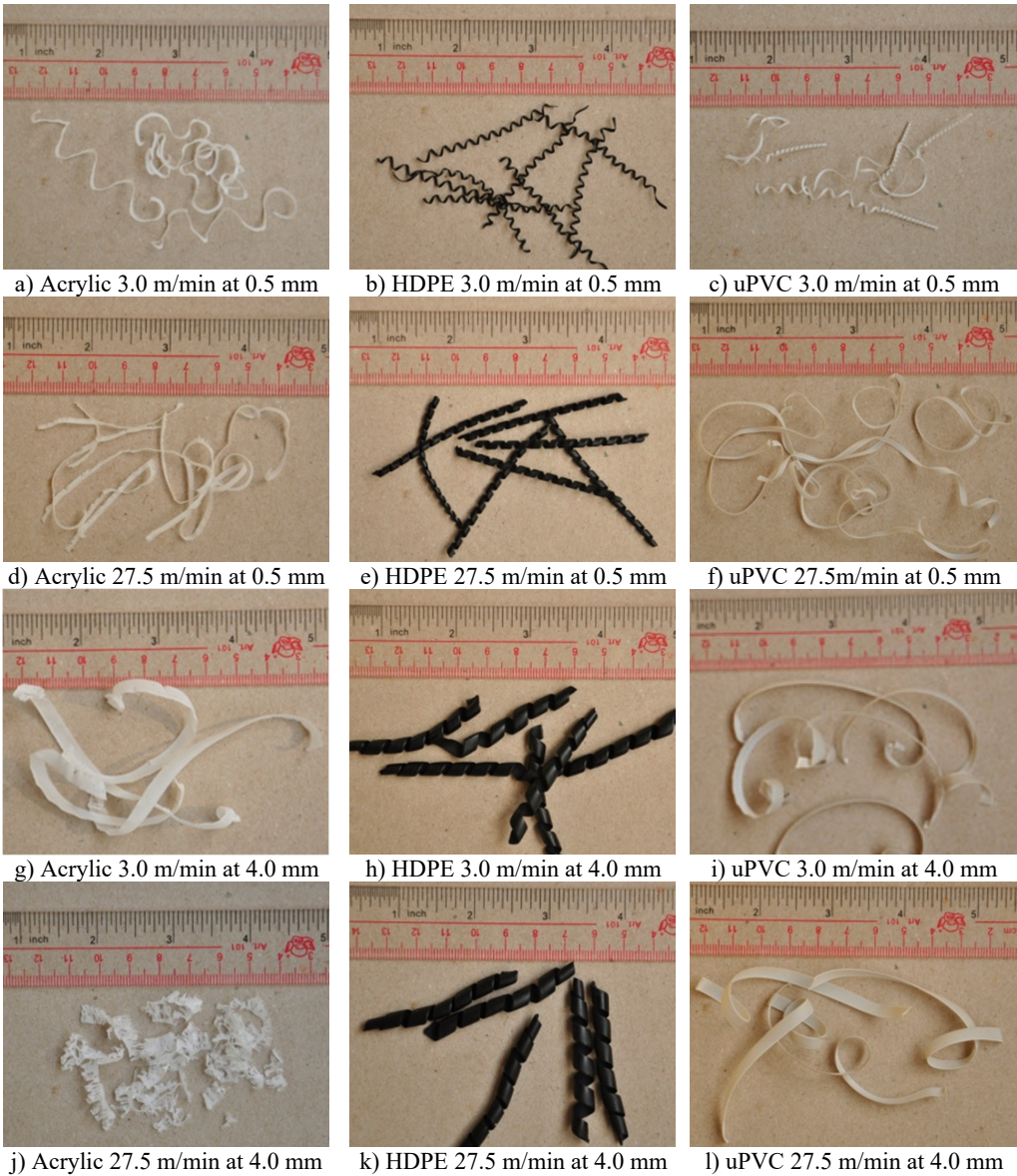
Fig. 8. Photo micrograph of the chips generated due to machining at different cutting speed and depth of cut
