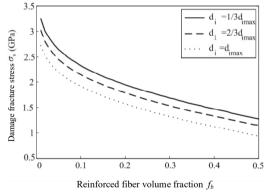
Fig. 3. Schematic representation of the variation of damage fracture stress with reinforced fiber volume fraction
