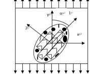
Fig. 1. Two scale cell model of eutectic with symmetrical triangular reinforced fibers
