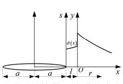
Fig. 4. Model of damage localization band at crack tip
