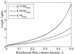
**Fig. 5.** Relationship between the length of damage localization band and reinforced fiber volume fraction
