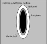
Fig. 2. Microcosmic cell and effective medium
