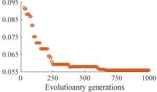
a) The fitness of the driver's seat vibration b) The fitness of the cab pitch vibration **Fig. 4.** The curve of fitness values of the AGA
