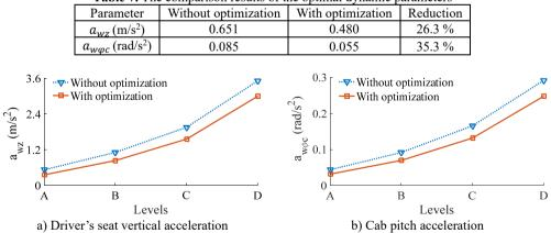
Fig. 6. Result of the weighted RMS accelerations of the cab and seat under various road surfaces
