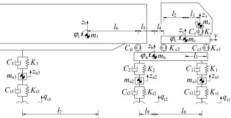
Fig. 1. Lumped parameter model of heavy trucks
