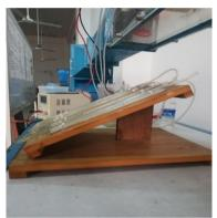
Fig. 3. Inclined manometer
