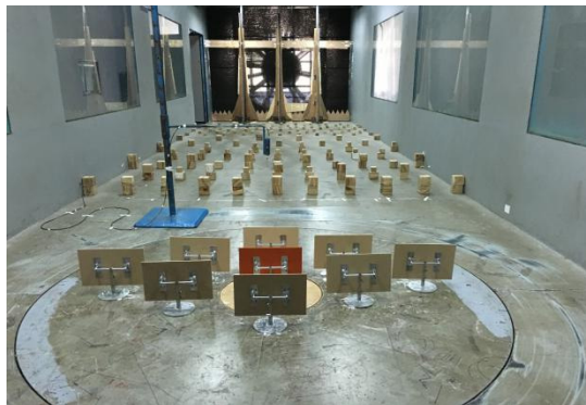
Fig. 1. Wind tunnel test of heliostats
