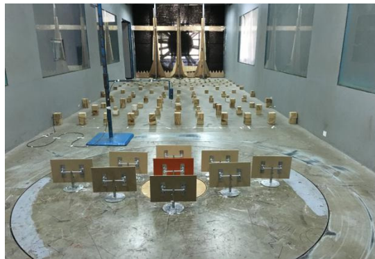
Fig. 1. Wind tunnel test of heliostats
