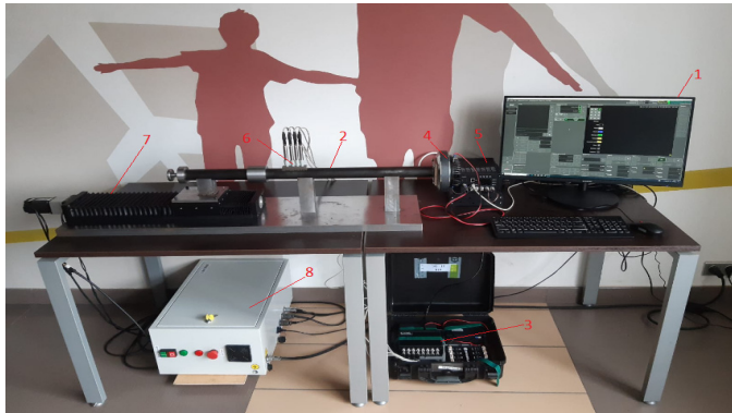
Fig. 1. General view of MAI interferometer installation (impedance tube) with normal incidence of sound waves for studying the acoustic characteristics of sound-absorbing materials and structures:
