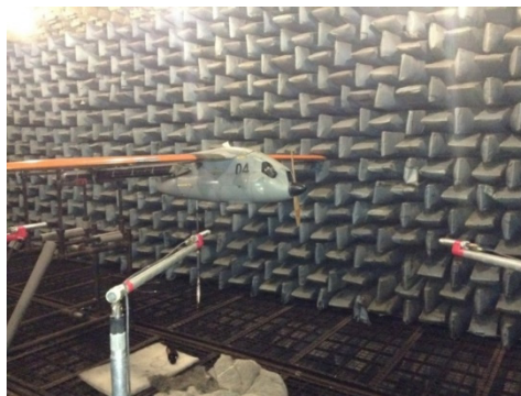
Fig. 2. Location of a Ptero-G0 UAV during testing in an anechoic chamber AC-2
