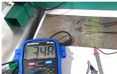
Fig. 7. Lateral and transvers strain gauges located at the rectangular plate surface
