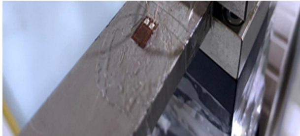
Fig. 5. Strain gauge located at the beam root
