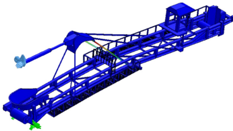
g) Frequency of the landing boom structure is 4.76 Hz, and deformation is 14.5 mm – lamella displacement
