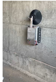
b) The wall-climbing robot equipped with a brush for cleaning
