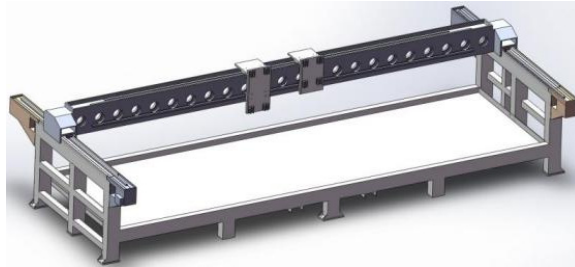
Fig. 1. Simplified model of the entire Double-head machine tool
