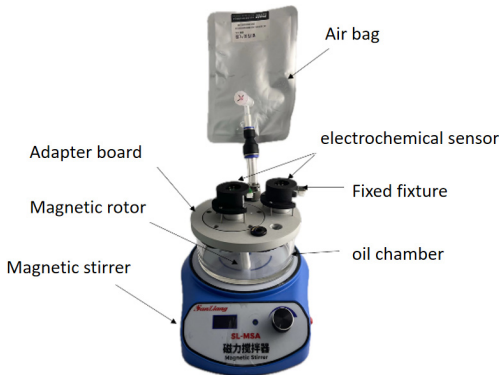
Fig. 8. Experimental setup for dissolved gas detection in oil
