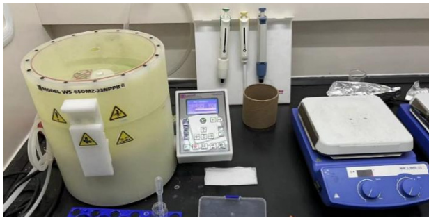
Fig. 1. Experimental setup for preparing hydrocarbon vapor separation membranes utilizing spin coating
