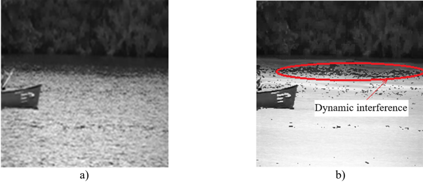
Fig. 3. Schematic diagram of the results of suppressing dynamic background: a) original image, b) result of suppressing dynamic background
