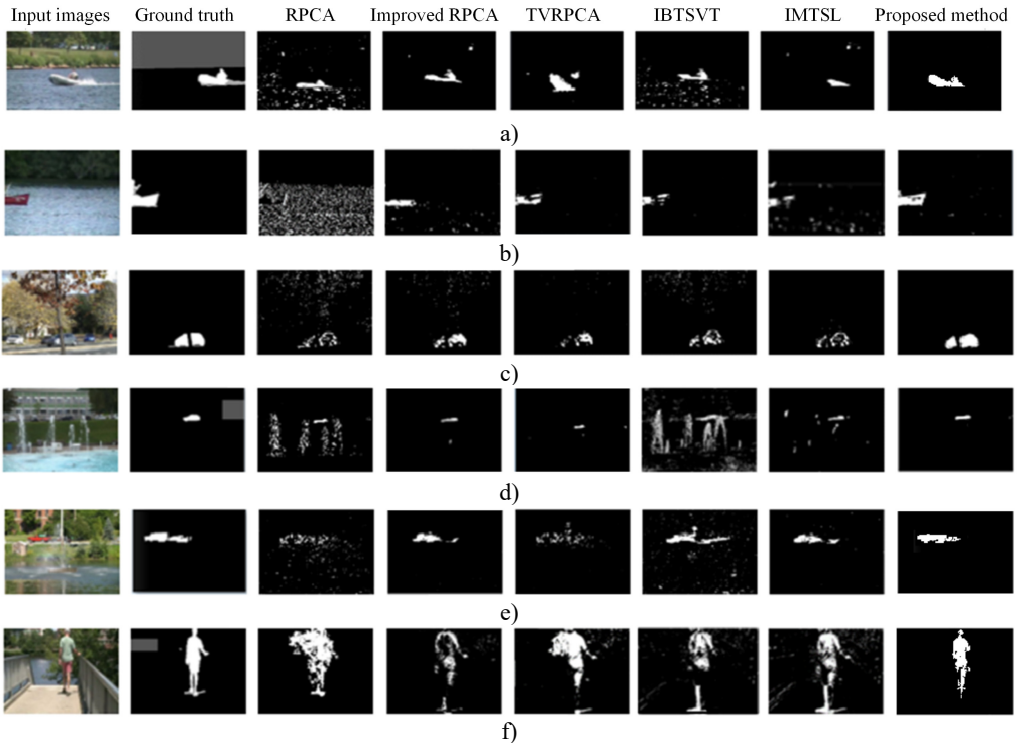
Fig. 8. Results of different algorithms for extracting moving targets: a) boats, b) canoe, c) fall, d) fountain01, e) fountain02, f) overpass
