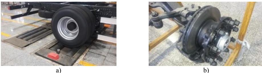
Fig. 1. Real model of the BD: a) brake test, b) assembled brake
