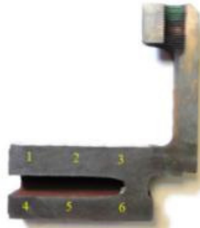
Fig. 10. Numbered position of damaged disc for hardness test
