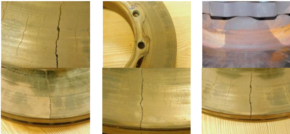
Fig. 6. Crack types on FD
