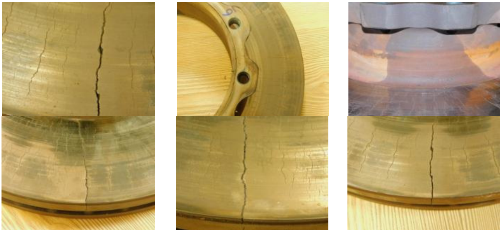
Fig. 6. Crack types on FD
