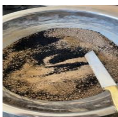
a) Loess mixed with rubber particles
