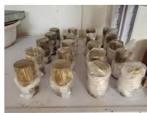
c) Post freeze-thaw specimen
