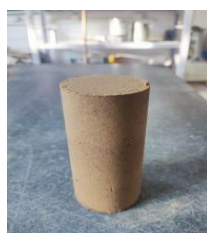
b) Triaxial specimen
