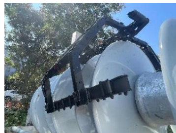
Fig. 1. Physical image of the insulator Electric field detection robot
