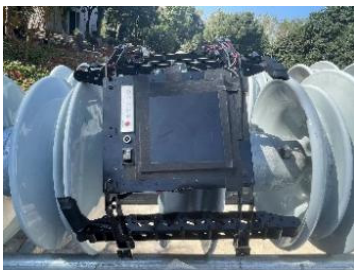
Fig. 1. Physical image of the insulator Electric field detection robot
