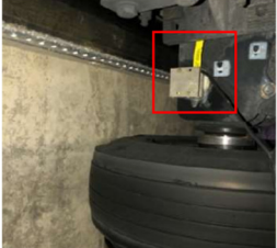
d) Stabilising wheel lateral displacement measurement point
