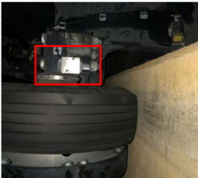
b) Guide wheel lateral displacement measurement point
