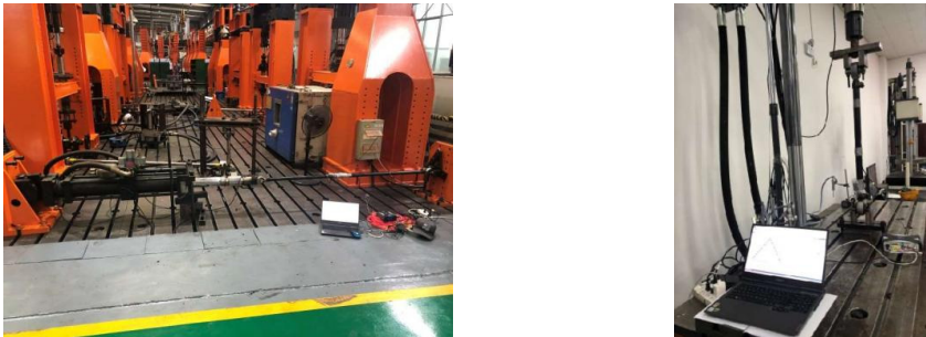
Fig. 3. Connecting rod calibration equipment
