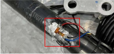
c) Longitudinal tie rod measurement point
