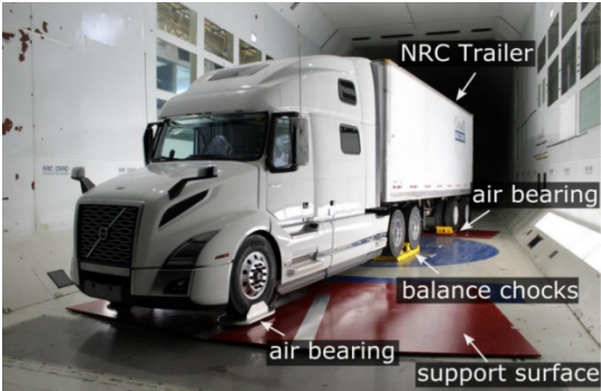
Fig. 1. Setup for the full-scale tractor-trailer wind tunnel experiment with the Volvo VNL860 tractor at a yaw angle of 10°
