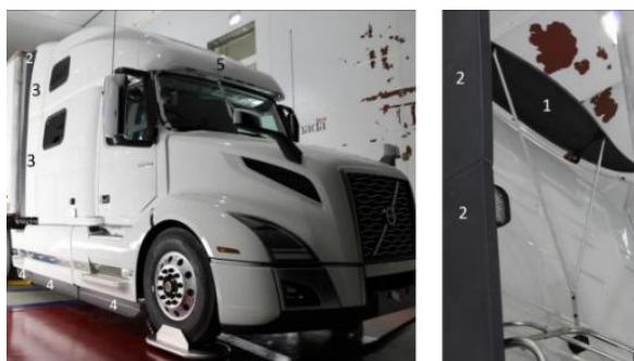
Fig. 2. Aerodynamic packages that were removed or installed during the test
