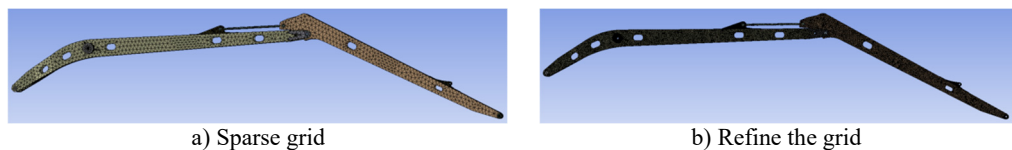
Fig. 2. Finite element model of the whole machine with different mesh densities
