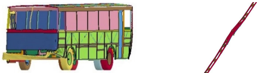
Fig. 13. Post-collision damage characteristics of medium bus and guardrails
