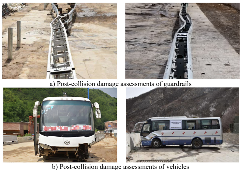
Fig. 21. Post-collision damage characteristics of guardrails and vehicles
