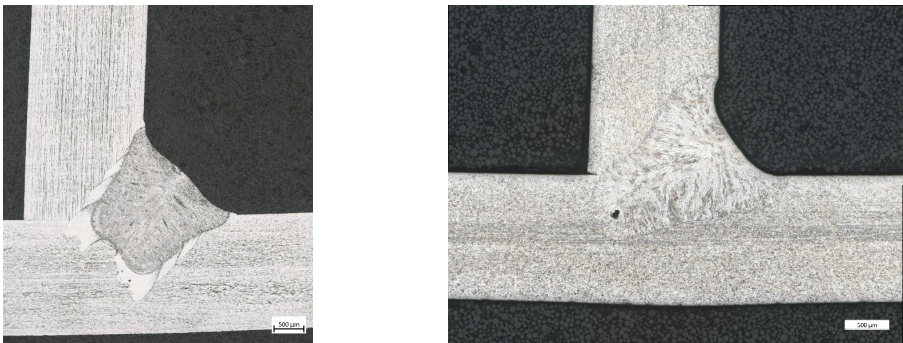
Fig. 8. Different T-joints done by HLBW [photos taken at ifw Jena, January 2024]
