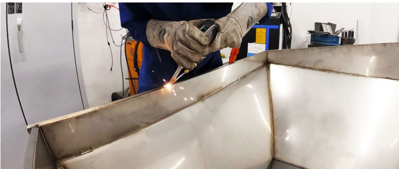
Fig. 10. HLBW welding of the stainless funnel made for winery [photo taken at ifw Jena, September 2023]
