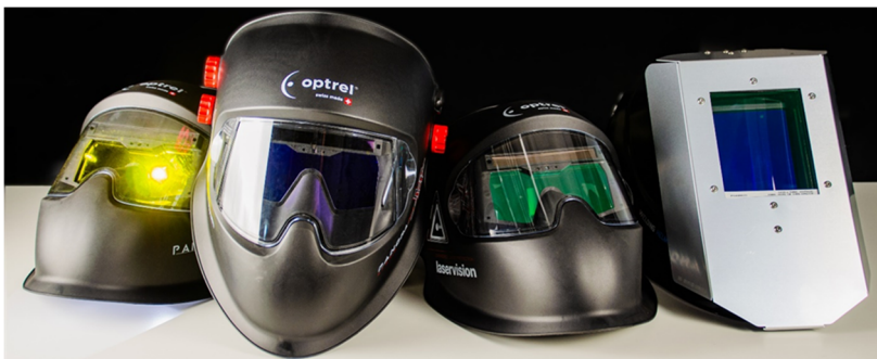
Fig. 6. Different helmets for HLBW [photo taken at ifw Jena, August 2024]
