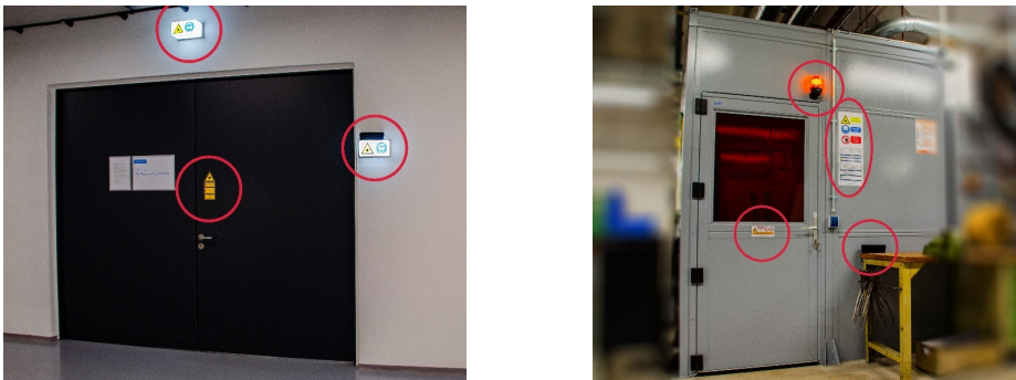
Fig. 7. Information about laser systems in use and signals for “laser on” outside the LCA [photos taken at ifw Jena, August 2024]
