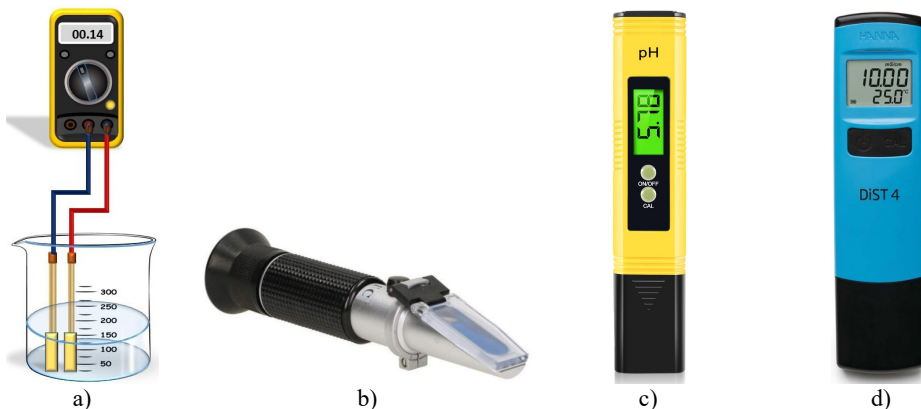
Fig. 1. Simple investigation of emulsion quality: a) simple investigation of liquid by resistance measurement with the multimeter and two electrodes, b) refractive index measurement refractometer, c) pH meter, d) conductivity tester
