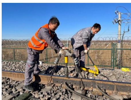
Fig. 6. Wheel-rail force calibration device
