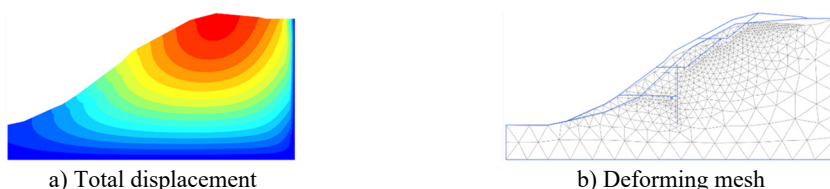
Fig. 4. Total displacement and deformation grid of natural slope
