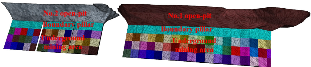
Fig. 7. Spatial relationship between the isolation layer and the open-pit and underground mining areas
