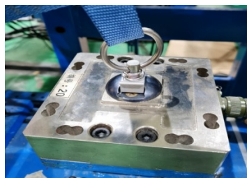
Fig. 6. Triaxial force sensors at constraint points
