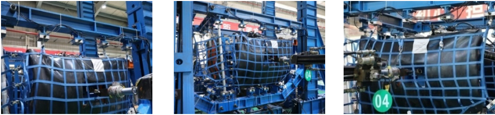
Fig. 7. Normal failure mode of the restraint net
