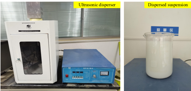
Fig. 3. Ultrasonic disperser and resulting suspension. Photo taken by Dr. Yapeng Wang on February 22th, 2024 at the Experimental Laboratory Building of Northwest Institute of Eco-Environment and Resources, Chinese Academy of Sciences
