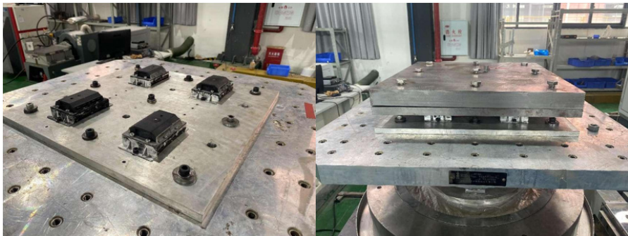
Fig. 6. Vibration isolation performance test of the vibration isolator
