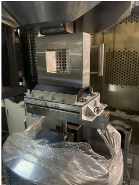
Fig. 4. The static stiffness test of the vibration isolator
