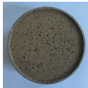
b) After collapsibility test (RPC = 5 %, RPS = 20 mesh)
