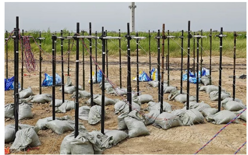
a) Installation status of ground-reflection pressure sensor b) Installation status of free-field pressure sensor Fig. 11. Sensor on-site installation status. Photo by Liangquan Wang during the research process
