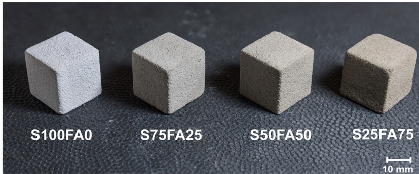
Fig. 6. Powder-based 3D printed green cubes using geopolymer powders with different slag/fly ash ratios [12]
