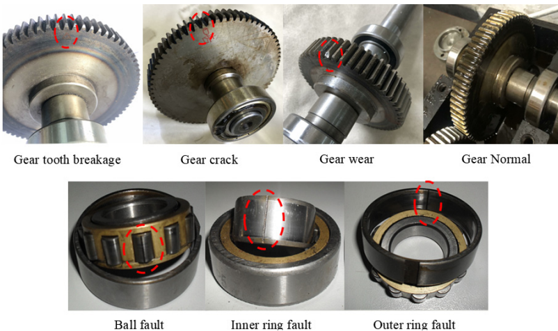
Fig. 6. Wind turbine bearing failure in different locations
