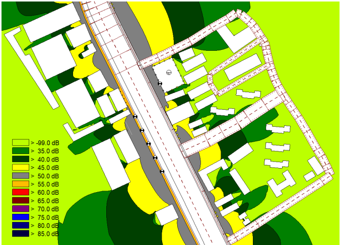
Fig. 5. Map of the night noise results of the Huangsha Avenue – Inner Ring Road Elevated Bridge with noise reduction measures in place
