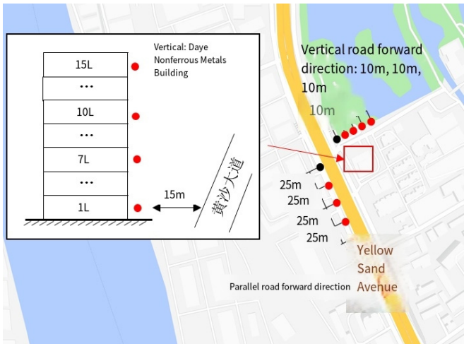
Fig. 1. Schematic diagram of the layout of measurement points on the Huangsha Avenue – Inner Ring Road elevated Bridge
