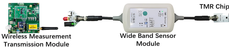
Fig. 5. Prototype of wideband current wireless measuring device
