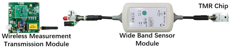
Fig. 5. Prototype of wideband current wireless measuring device
