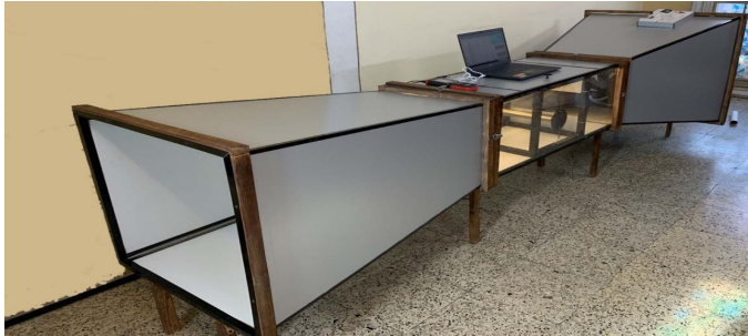
Fig. 2. The actual open wind tunnel. The Figure captured by Dr. Firas Ali Jasim, on 12 December 2023, at the home workshop in Iraq
