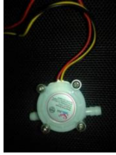
Fig. 10. The physical picture of turbine flowmeter. Photo by Yuli Ouyan, Southwest University, Chongqing, May 2025
