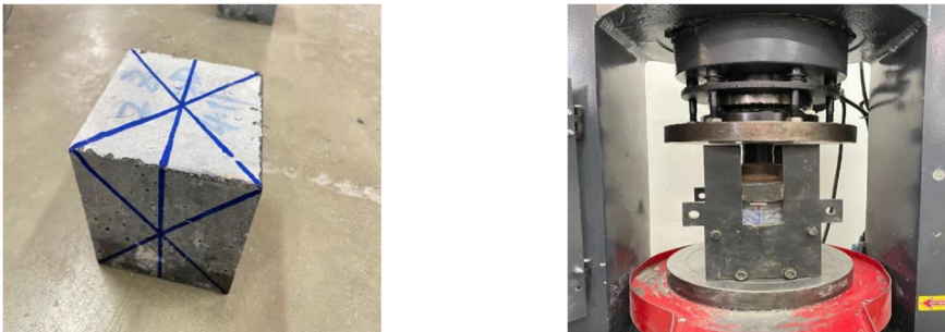
Fig. 1. Splitting strength test (Hanghang Wang took the photo, Chang'an University, and 2025.06.03)
