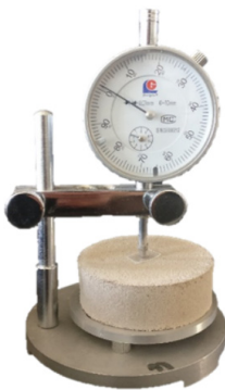
a) Set-up of contractometer SS-1
