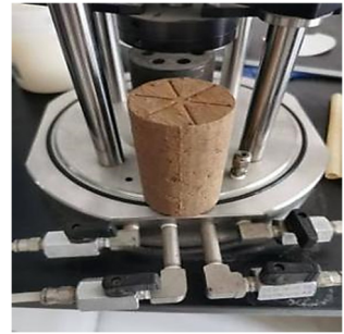
c) Soil triaxial experiment
