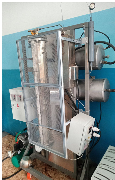
Fig. 2. General view of the laboratory unit for oxidative-reductive regeneration of spent zeolites. The photograph was taken in March-April 2024 at “Neftgazinnovatsiya” LLC, Tashkent, Uzbekistan, where the prototype of the industrial-scale installation was developed
