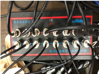
b) Eddy current sensor conditioner
