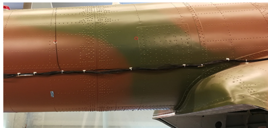
Fig. 15. Transmission sensors cable harness (A. Safonovs, 20.09.2025, Tbilisi)
